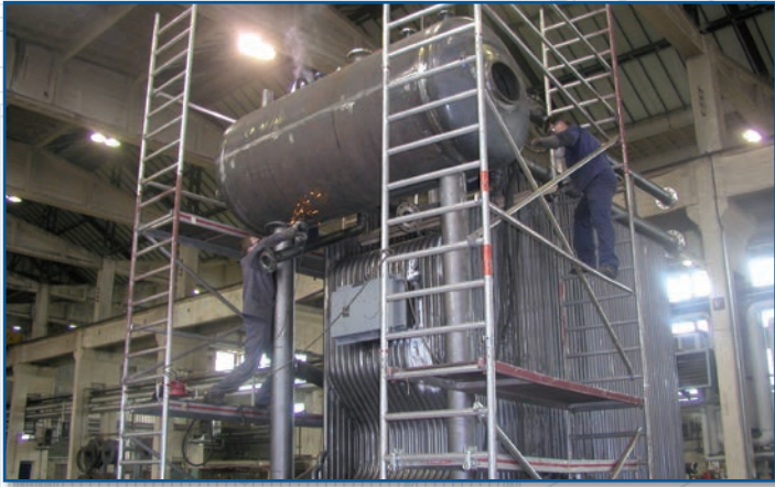
Watertube boiler during manufacturing
