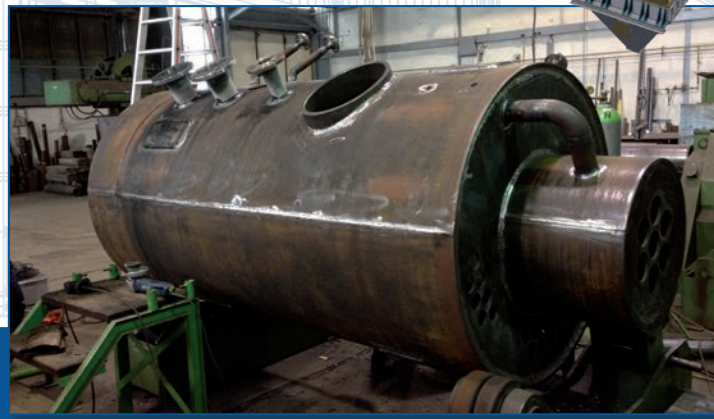
Small smoketube waste heat boiler during assembly
